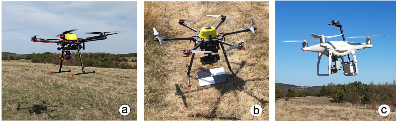
Figure 2. UAVs platforms: (a, b) Tarot X6 hexacopter; (c) DJI Phantom 4 Pro with installed PPK-GNSS kit.
