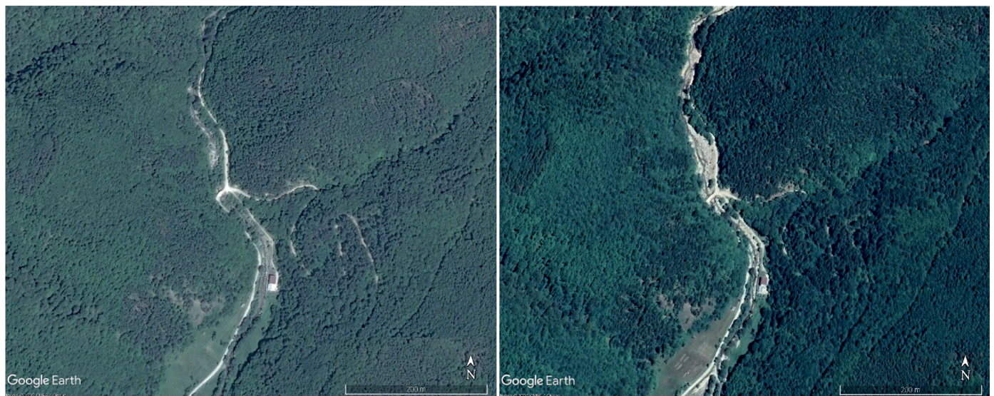
Figure 3. Formation of new river channels at the expense of the flood plain and newly formed cobble-boulder accumulations during mid 2019 flash flood event. Location: next to the Cherna Mesta powerplant (visible on the lower central part).
